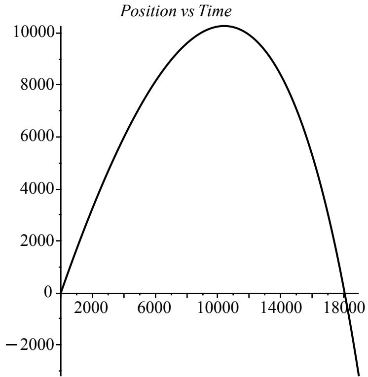
Notice the air resistance effect. This plot is not a parabola now.
