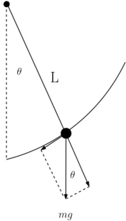
The primary forces are gravity that make it move when pulled away from its rest position and the force (tension) in the rod to keep it moving along a circular path. It also may have a damping force due to friction.
