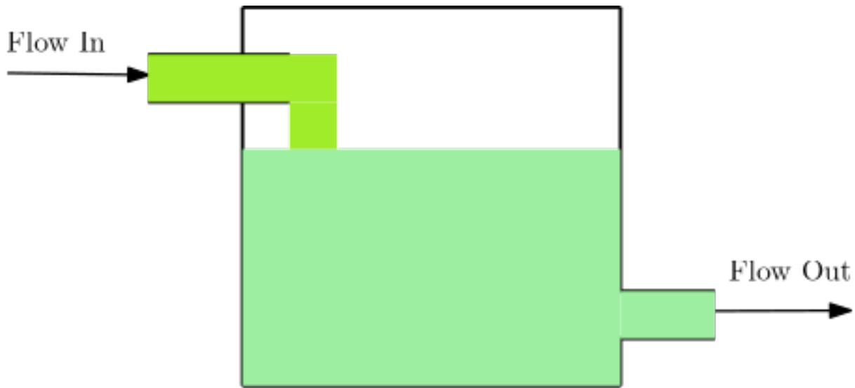
Now, it is the rate of change of salt present in the tank that we want to understand. Let the amount of salt dissolved in the tank at any point in time be  $A(t)$ . We are then interested in the rate of change of  $A$  or
